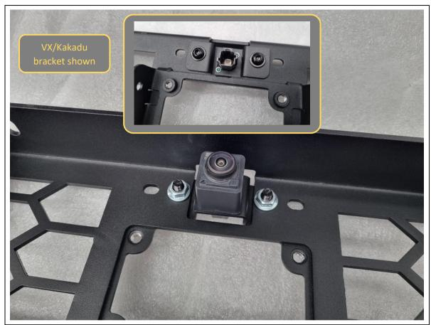
164. Fit the camera and bracket from the back of the centre mesh, and secure with 2x M6x16 black button head bolts, black washers and flange nuts.
