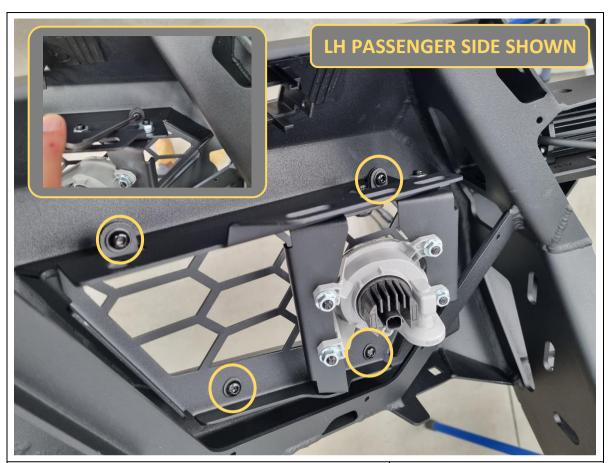
96. Fit the wing meshes with lights to the inside of the bull bar wings. Secure each wing mesh with 4x M6x16 black button head bolts and black washers, into the embedded nuts in the bull bar.
