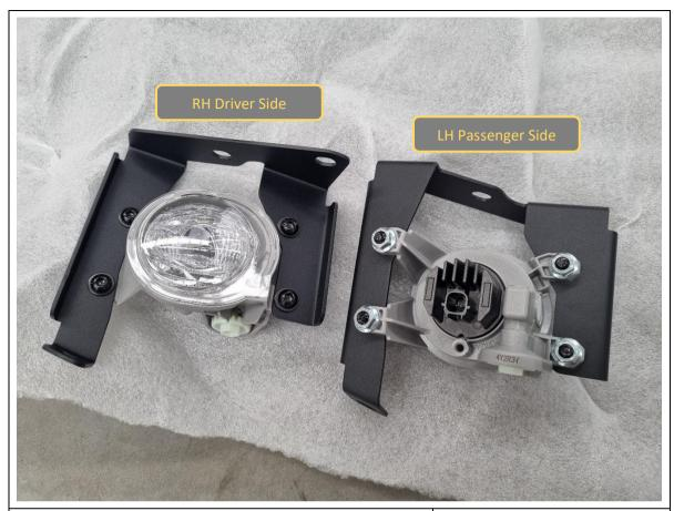
90. The original fog lights can be re-fitted to the bar. Fit the fog lights to the supplied B-1431 fog light brackets and secure with 4x M6x16 black button head bolts, black washers and flange nuts, each.
