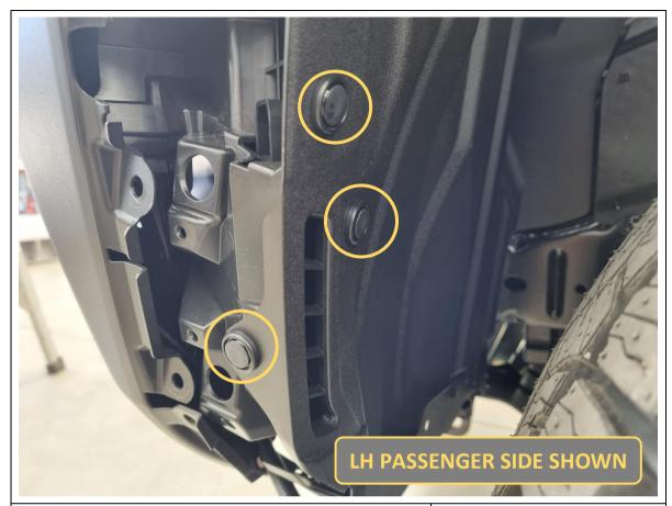
15. Remove 3x plastic push clips holding the front of the inner wheel guard. Do this on both sides.
