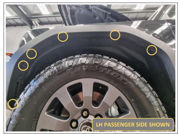
9. Remove 5x plastic push clips and 1x 10mm hex screw holding each front flare.
