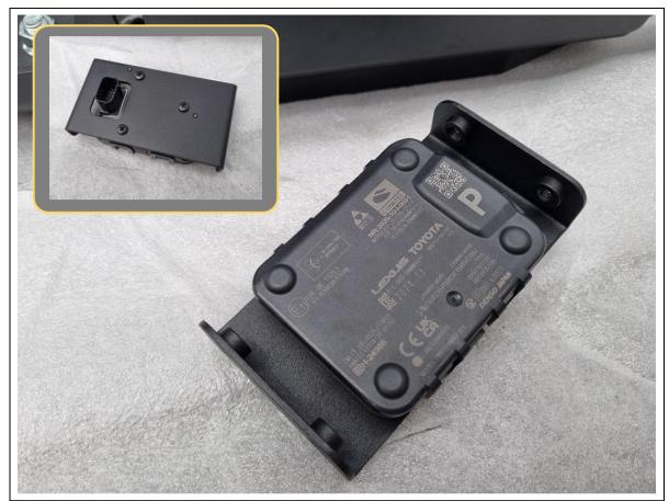
167. Re-fit the radar to the supplied B-1447 relocation bracket and secure using the retained screws.
