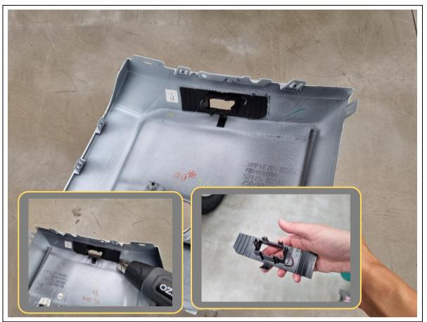
79. Use a combination of heat gun, plastic trim tool and utility knife to peel off the headlight washer holders from each bumper insert.
