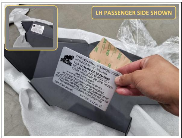
199. Peel off the backing film and affix the ADR compliance plate to the inside of the LH side underpanel.
