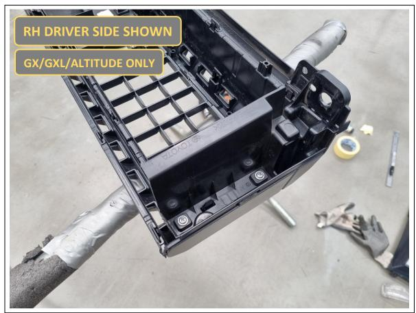
136. **GX/GXL/Altitude only.** Re-fit the plastic grille side retainers to the grille using 2x Phillips head screws, each.
