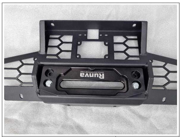
160. If fitting a winch, fit the hawse fairlead to the centre mesh now using M10 or 3/8" fasteners supplied with the winch. This bar is only compatible with hawse type fairleads.
