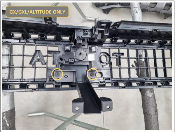
137. **GX/GXL/Altitude only.** Fit the B-1452 grille support to the back of the grille, where the radar was mounted. Re-use the 2x 10mm hex bolts from the radar.
