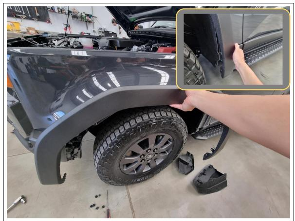
10. Starting from each end, pull the flare outwards and release the 14x body clips holding it to the body. Set the flares aside in a safe place for later.
