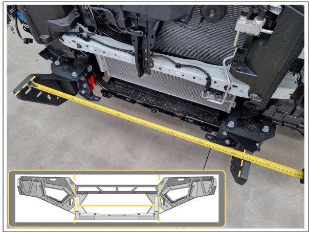
50. Measure the distance between the outside faces of the uprights on the bull bar using a tape measure. Write the distance below for reference if required:
