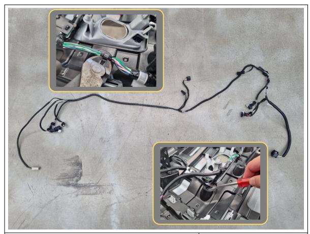
66. Fully strip the bumper wiring harness off the bumper by either unclipping the harness with a flat blade screwdriver or trim tool, or by carefully cutting off the cable tie clips with side cutters (take care not to cut the wires).
