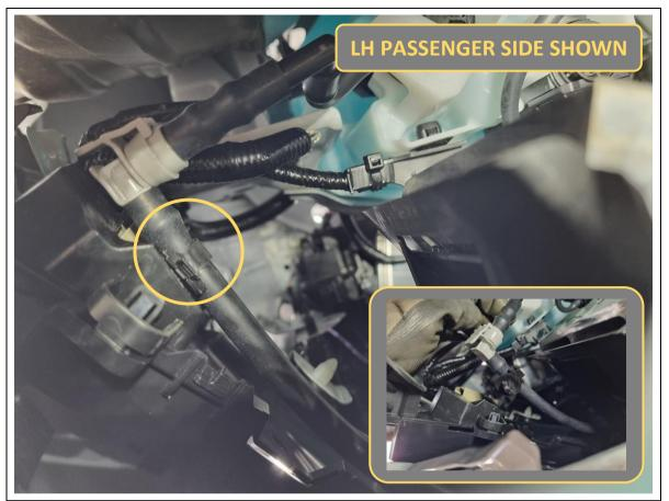
19. On the passenger side, there is a headlight washer hose that is clipped into the bumper in one location. Unclip the hose.
