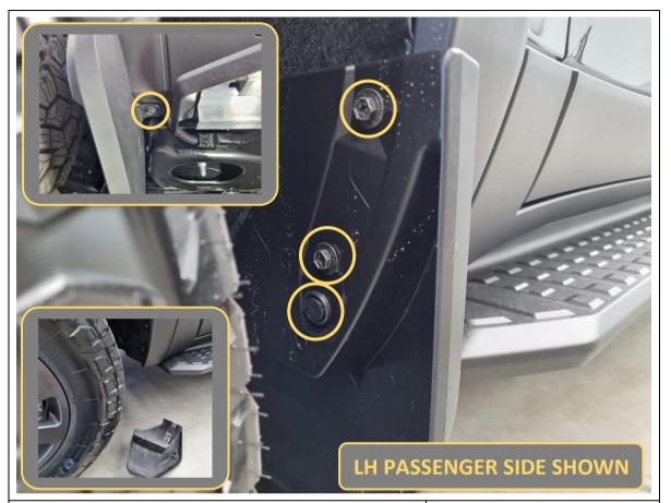
8. The front flares and mudflap need to be removed. Start by removing 3x 10mm hex screws and 1x plastic push clip holding each front wheel mudflap.
