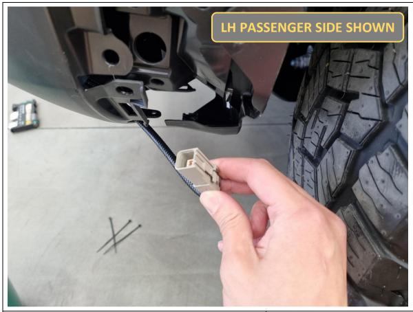
18. On the passenger side, do the same and disconnect 1x bumper harness connector. This connector has a single unlocking tab that can be pressed down with a thumb.
