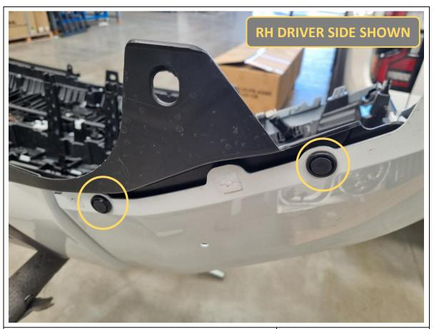
73. Remove 2x plastic push clips on the bottom of the outer bumper extension. Do this for both sides.
