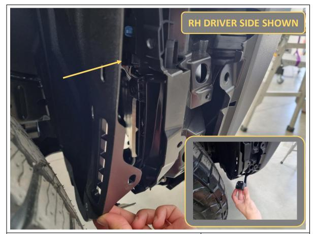
17. On the driver side, pull back on the inner wheel guard to gain access inside, then disconnect 1x bumper harness connector.
