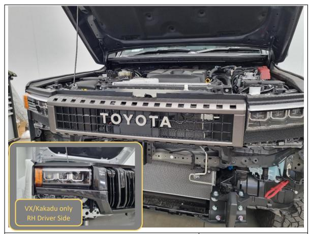
139. Re-fit the grille back onto the vehicle.
