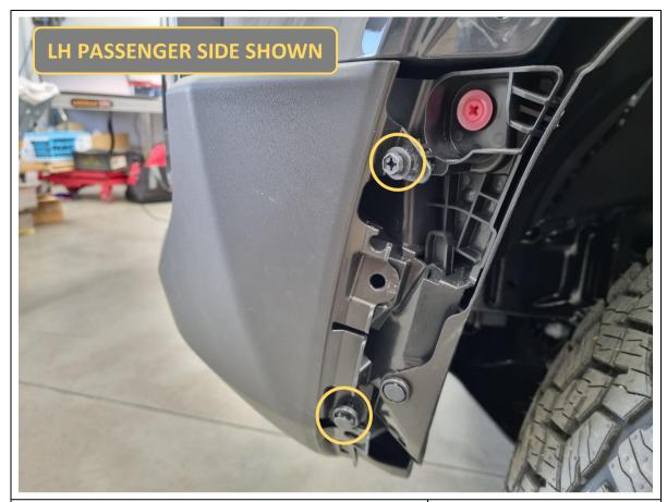
14. Remove 1x 10mm hex bolt and 1x plastic push clip on the outer end of the bumper. Do this on both sides.
