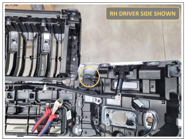
64. On the driver side of the bumper, unclip the blanking plug highlighted. Use a flat blade screwdriver or trim tool to assist.
