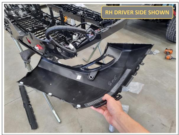
75. Release 3x tabs to remove the outer bumper extension. Do this for both sides.
