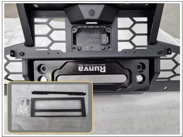
Locate the number plate flip brackets and fastener kit.
