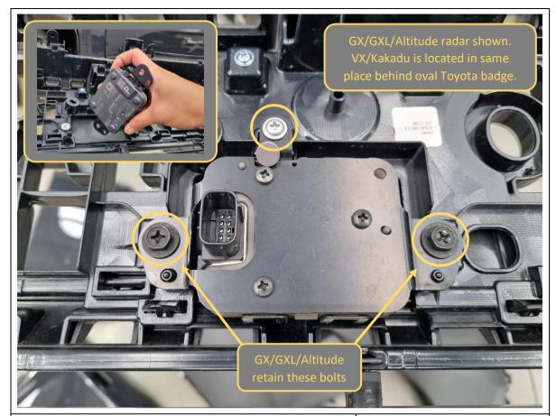
The radar and camera need to be removed before the grille goes back on the car.
