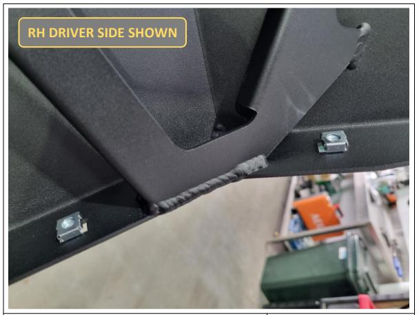
58. Fit 10x M6 cage nuts into the rectangular slots in bottom of wing (5x per side).
