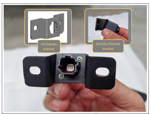
163. Fit the camera to the supplied camera bracket and secure with the same T6 Torx screws. The cutout in the bracket is keyed, so the camera can only be fitted in one way.
