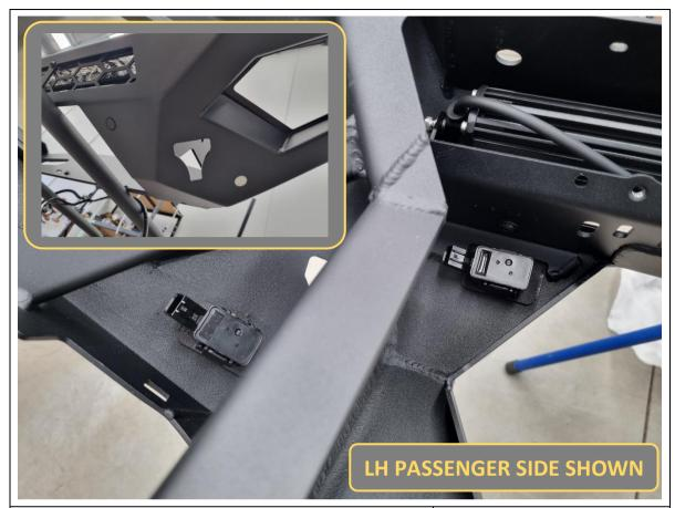
87. Remove the backing film off the tape on the parking sensor holders (use utility knife or 90 degree pick to assist), then fit to their corresponding positions inside the bull bar.
