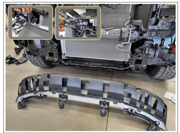
31. Remove 8x 17mm hex bolts (4x per side) holding the crash beam to the chassis.
