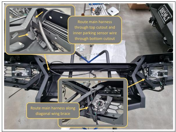
103. Route the bumper wiring harness through the bar and connect the fog lights and parking sensors.
