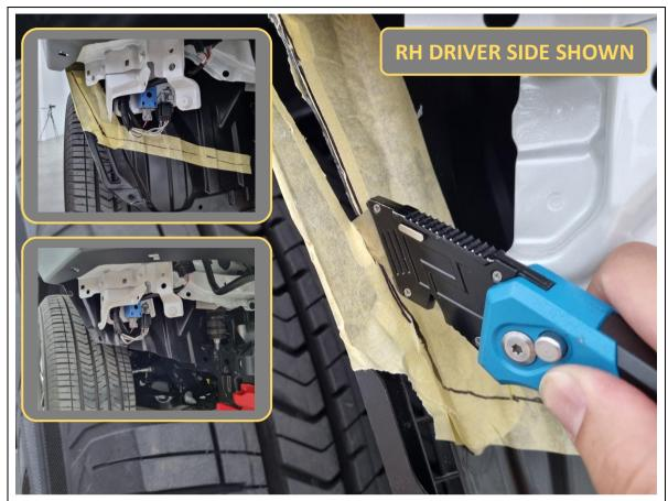
203. Remove the side underpanels, then cut the wheel arch liners along the marked lines using a utility knife or similar cutting tool.
