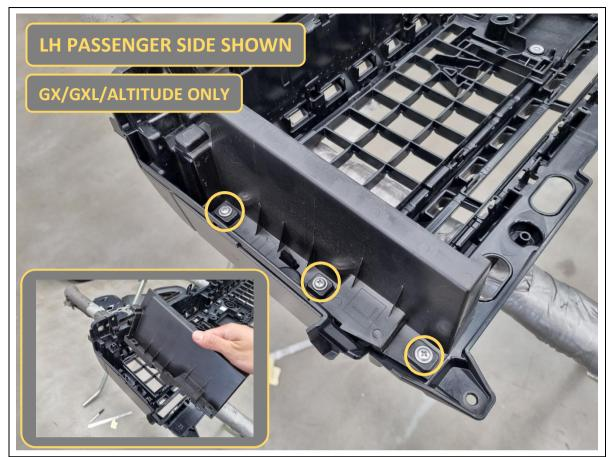
129. **GX/GXL/Altitude.** Remove 3x Phillips head screws holding each plastic grille side retainer. Retain screws for re-assembly.
