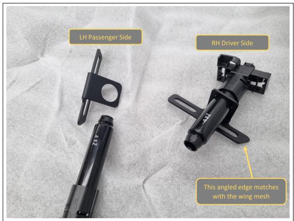
99. Slide the B-1465 headlight washer retainer brackets onto the main shaft of the headlight washer units.
