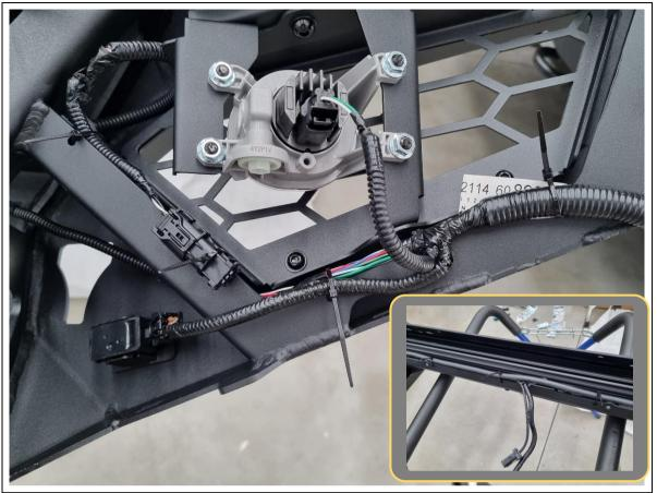
105. Secure the bumper wiring harness and washer hose to the provided holes in the bull bar using cable ties.
