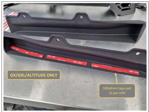
Allow at least 5 minutes for the primer to chemically bond to the surfaces before applying tape.
