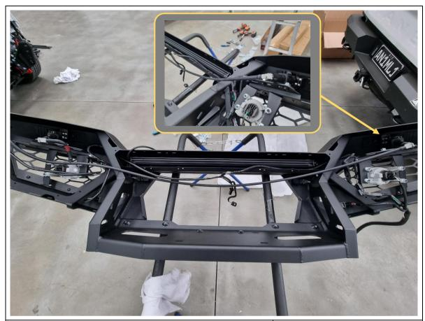
104. Connect the washer hose back to the headlight washer units. Leave the washer hose sitting on the outside of the bull bar, do not route through the cutouts inside.
