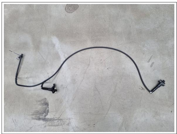
72. Either unclip or cut through the cable tie clips securing the washer hose system to the bumper and set aside.
