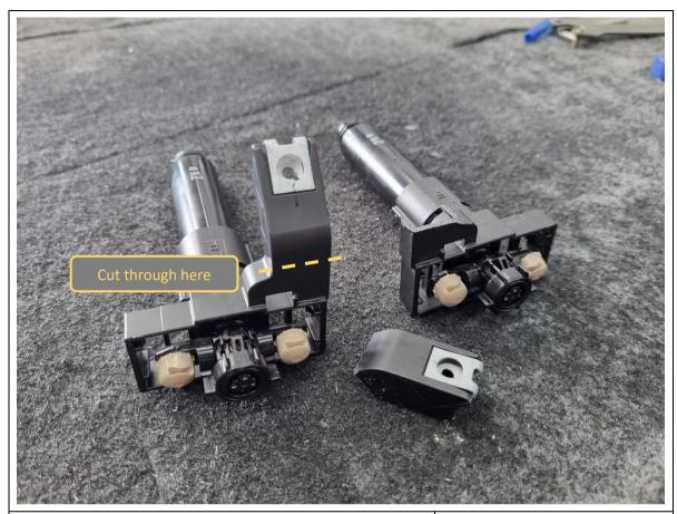
98. Using an air hacksaw or similar cutting tool, cut off the flange on each of the headlight washer units as shown. Ensure the washer unit is secured firmly (eg. with a table clamp) before cutting.
