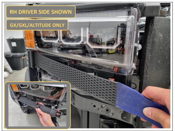
138. **GX/GXL/Altitude only.** Using a trim tool to assist, unclip the plastic under headlight trims, starting from the inner corner.
