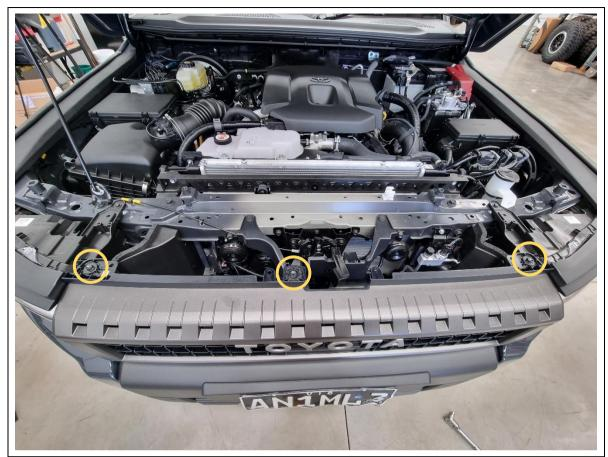
12. Remove 3x 10mm hex bolts holding the top of the grille.
