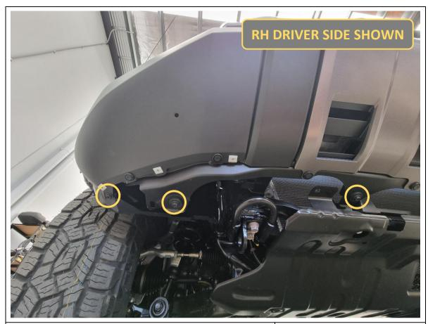
13. Remove 6x 10mm hex bolts (3x per side) holding the bottom of the bumper.
