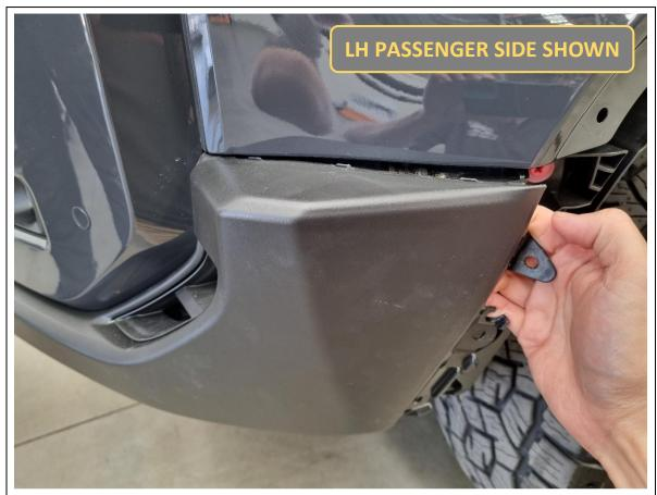
16. Grab onto each outer end of the bumper and pull outwards to unclip the outer section only. Do not unclip the rest of the bumper yet.
