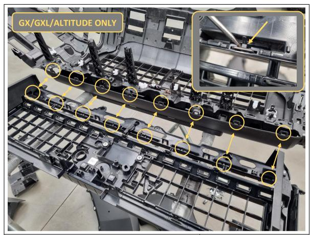
128. **GX/GXL/Altitude only.** Using a flat blade screwdriver or trim tool, release 8x tabs/clips holding the grille to the bumper. Fully separate the grille from the bumper. The bumper may now be discarded.
