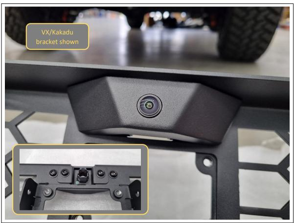
165. Fit the supplied camera housing to the outside of the centre mesh and camera, and secure from the back with 2x M6x16 black button head bolts and black washers.
