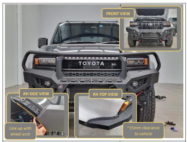
154. With assistance, from another person, align the bar with the edges of the vehicle. Adjust such that the clearances are neat, and the bar is symmetric left/right on the vehicle.
