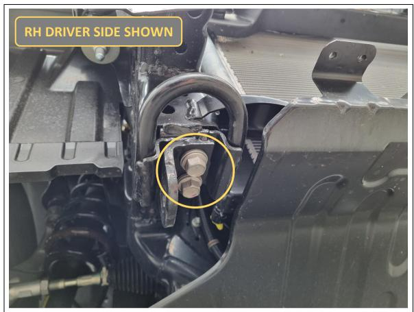
38. On the underside of the chassis, remove 2x 17mm hex bolts holding each tie-down point.
