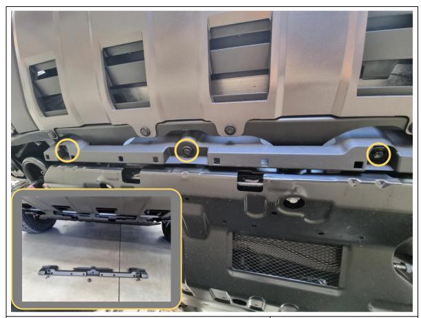
7. Remove 2x 10mm hex bolts and 1x plastic push clip in the centre holding the bottom bumper cover on the underside of the bumper.
