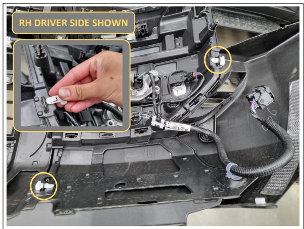
74. Remove 2x white plastic clips on the inside of the outer bumper extension. Do this for both sides.
