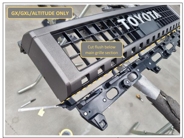
130. **GX/GXL/Altitude only.** The lower portion of the grille needs to be cut off. Mark out a cut line as shown. It will be flush with the bottom of the main grille section.
