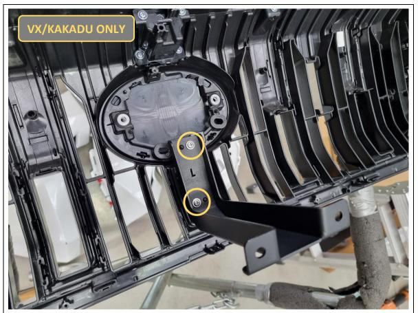
126. **VX/Kakadu only.** Fit the B-1469 grille support to the back of the grille, where the camera was mounted. Re-use the 2x Phillips head screws from the camera.
