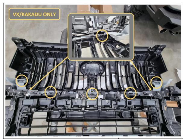
123. **VX/Kakadu only.** Using a flat blade screwdriver or trim tool, release 7x tabs/clips holding the grille to the bumper.
