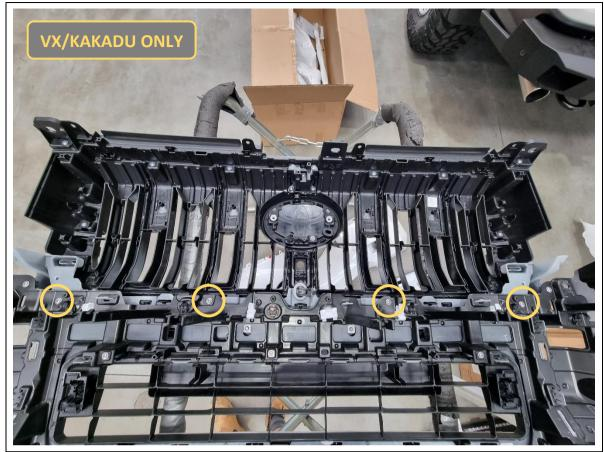
122. **VX/Kakadu only.** Remove 4x Phillips head screws holding the bottom of the grille to the bumper.
