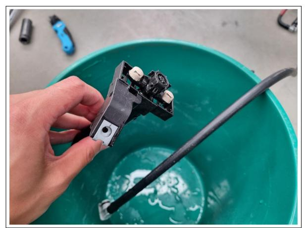
97. Disconnect the headlight washer units from the washer hose. Do this with a bucket as there will be some fluid spilling out.
