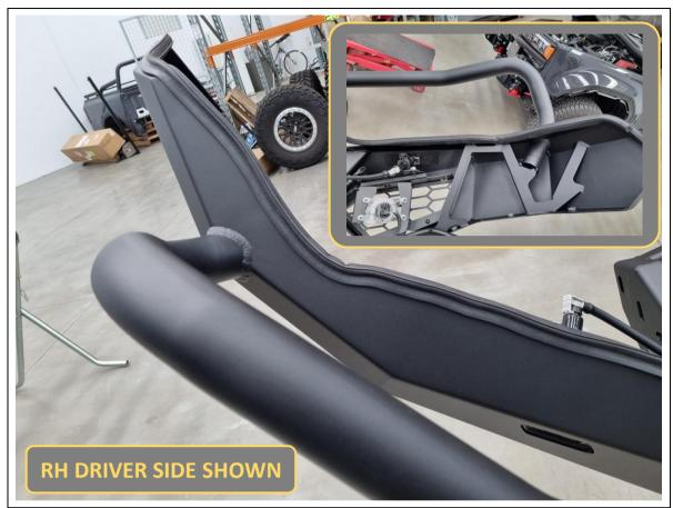
111. Fit the supplied 2x lengths of pinch weld rubber to the top edge of the bull bar wings. Trim off any excess around the centre section.
