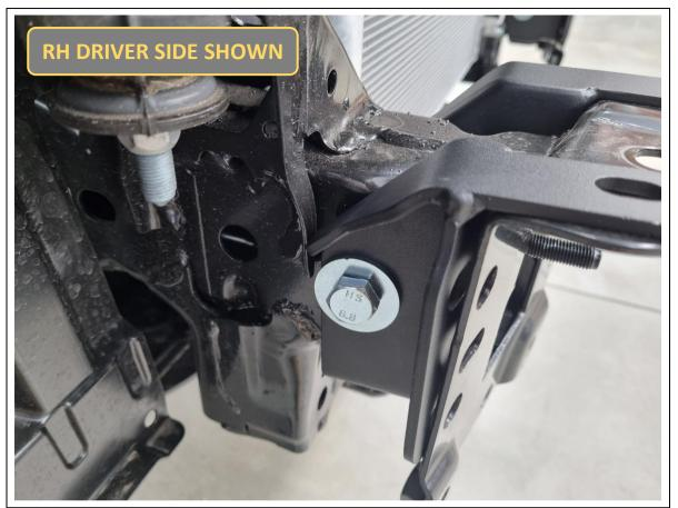
43. Fit the B-1142 outer chassis support brackets to the outside of each chassis rail, and secure/align in the same manner as the inner chassis support brackets.
