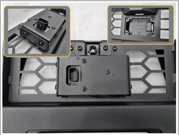
168. Fit the radar and relocation bracket to the back of the centre mesh, and loosely secure with 4x M6x16 black button head bolts and black washers.
