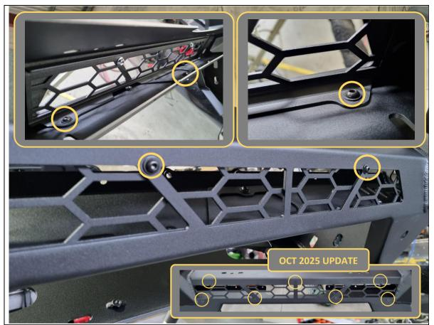
54. Fit the B-1434 light bar mesh infill to the inside of centre section the bull bar. Insert the middle tab in the bar first, then rotate to get the rest of the mesh in
