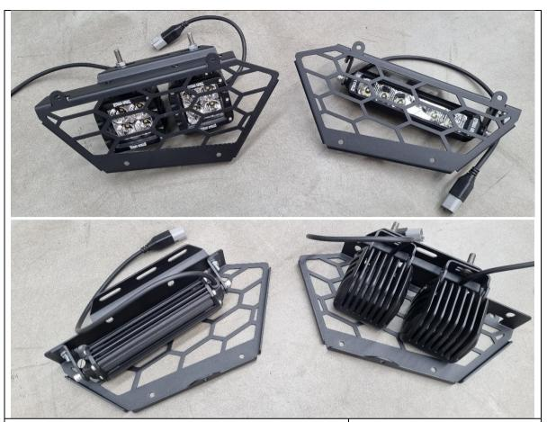
95. Instead of fog lights, there is also the option to fit an 8" light bar or up to two 2"x2" cube lights in each wing mesh, as shown. Or you can fit no lights at all.
