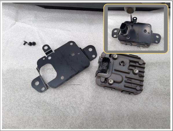
166. Separate the radar from its mounting bracket by removing 3x Phillips head screws. Retain the screws.
