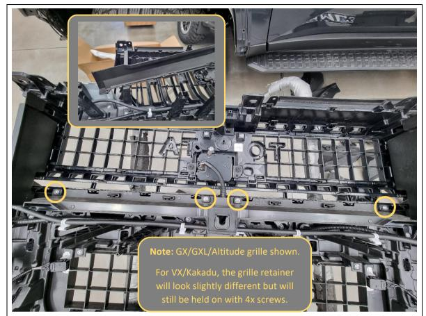
65. Remove 4x Phillips head screws holding the lower grille retainer.
